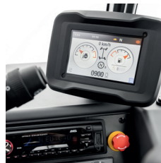
Standard 5" display with Bluetooth radio, microphone, & loudspeakers
