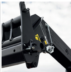
Hydraulic attachment lock using a dedicated auxiliary line
