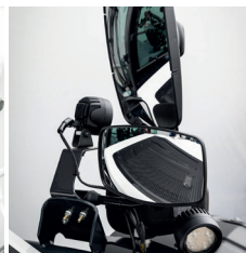
Electric mirror with de-icing on right-hand side
